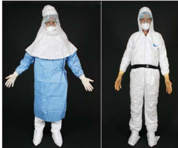
Fig. 2: The other system studied, named for its powered air-purifying respirator (PAPR), has 2 protective layers, shown above. The outer layer (left panel) consists of a hood, fluid-resistant surgical gown, shoe covers and 2 pairs of fitted surgical gloves. The inner (right) includes a hooded coverall and shoe covers, PAPR power unit, N95 mask, goggles, bouffant hair cover, and 1 pair of fitted surgical gloves. Contamination assessment for this layer was performed with the PAPR power unit and fitted surgical gloves removed. The towel worn to protect the neck has been omitted for illustrative purposes.
